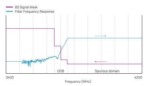
Fig 3 Illustration of the relationship between a 5G emission profile (BEM), and an RF filter response.
